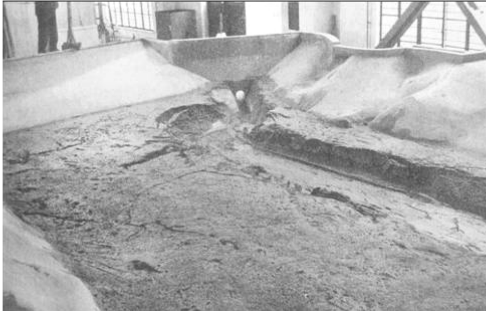
FIGURE 11.11 Physical model at 1:50 scale used to simulate the formation of a flushing channel using an 8m diameter low-level outlet at the Changma Dam on Shule River in the Gobi Desert. Model constructed by the Northwest Hydrotechnical Science Research Institute under contract to Gansu Provincial Government, China (G. Morris)
