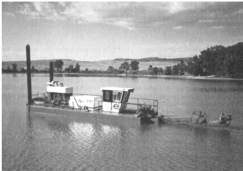
FIGURE 16.2 Photograph of a 25-cm hydraulic dredge with the cutterhead raised ( courtesy Ellicott International ).
